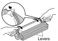
The toner cartridge is installed when the triangles match.
